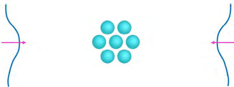
Figure 3-9: Unit Cell of a hexagonal photonic crystal placed in a dual counter propagating Gaussian Beam. The centered array is aligned with the beam axis. Particle radius: 0.5\mu\text{m} .
