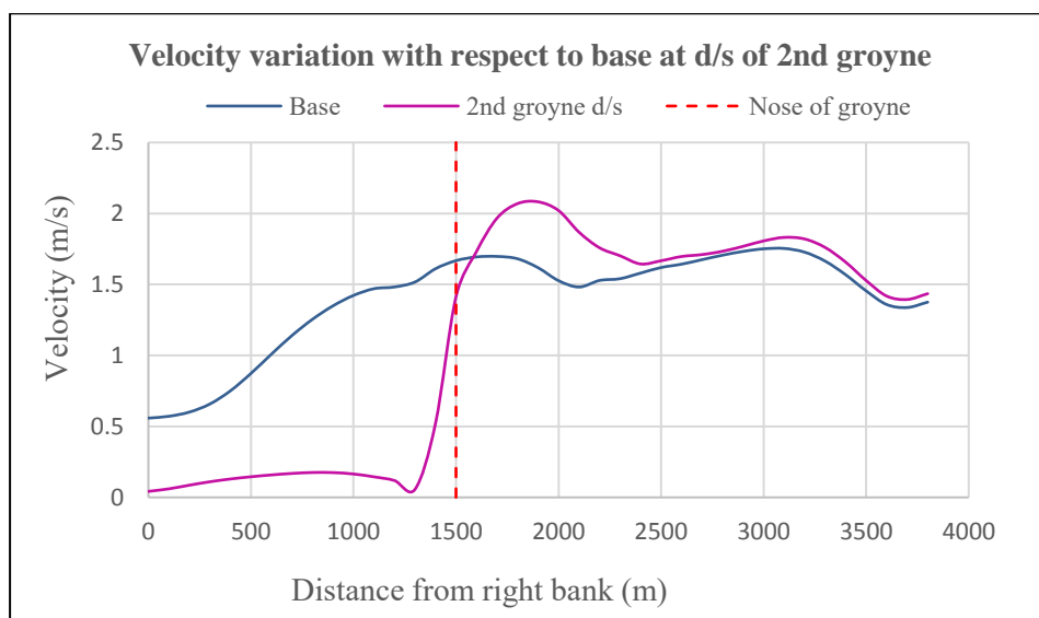
Figure 6.12: Comparison of velocity with base at the d/s of 2 nd groyne for option 2
