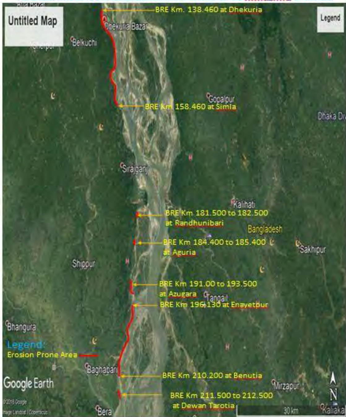
Figure 5.16: Erosion prone areas at the right bank of the Jamuna River
