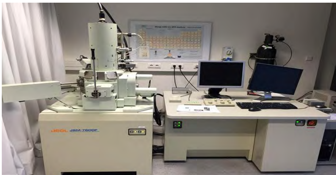
Fig. 3.7: JEOL JSM 7600F Scanning Electron Microscope
