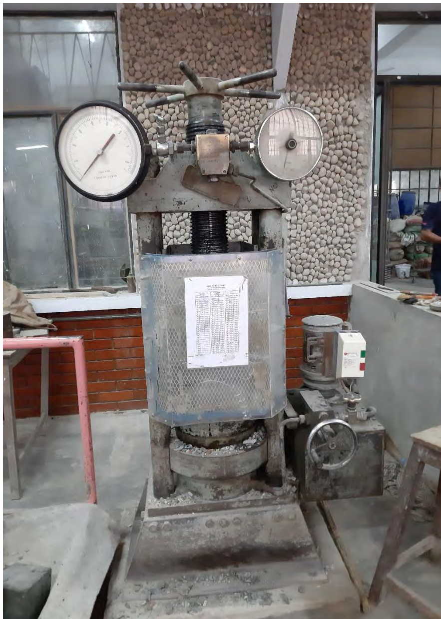
Fig. 3.10: Compressive strength testing machine for bricks
