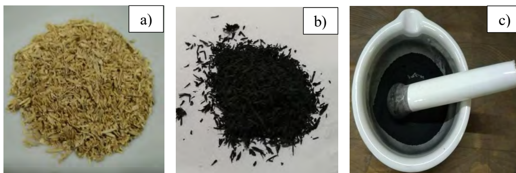
Figure 3.5: a) Dry RH before pyrolysis, b) rice husk biochar (RHB) c) Grinding of RHB
