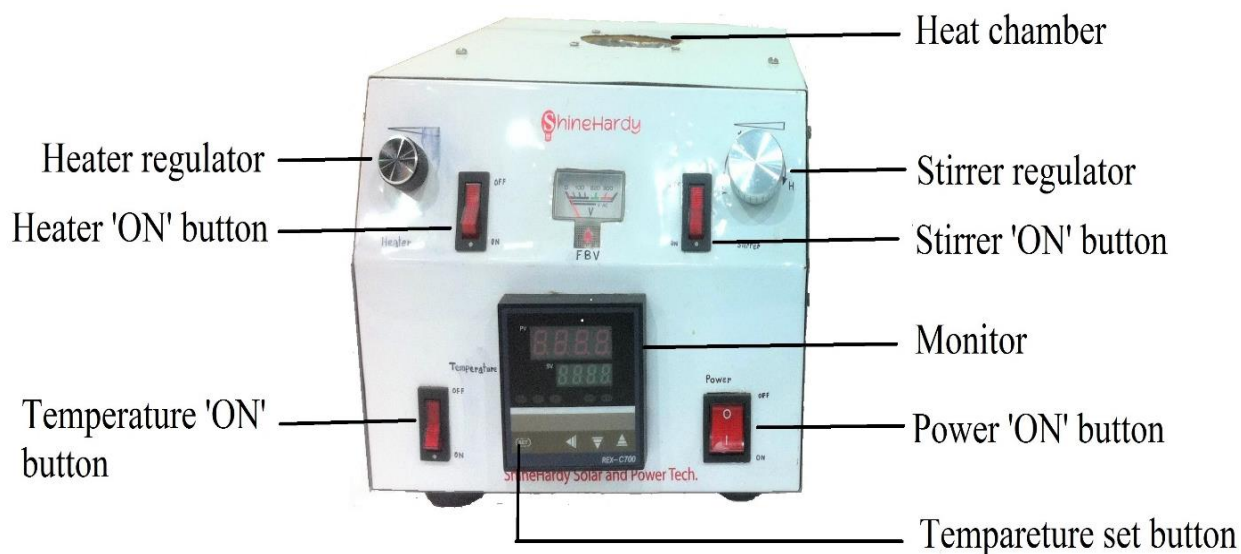
Figure 4.2: Locally fabricated chemical bath deposition unit at the Dept. of Physics, BUET
