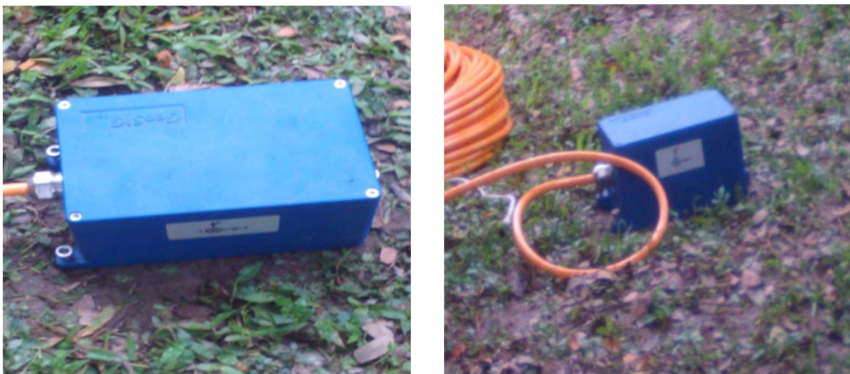
Figure 3.3: Microtremor testing equipment.
