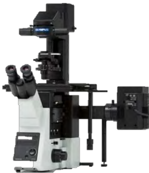
Fig. 3.19 Observation of GUVs suspension under Inverted phase contrast microscope (IX-73)
