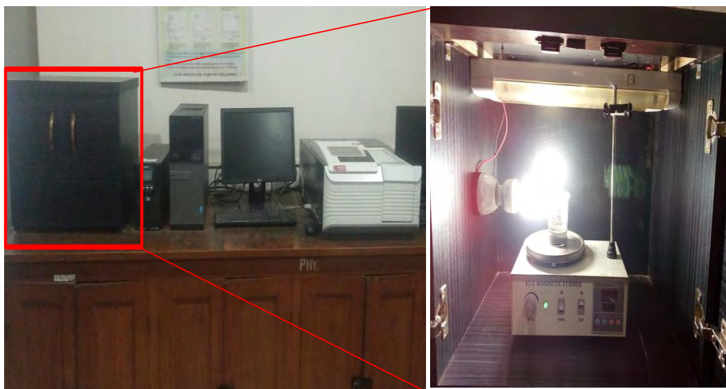
Fig. 21: Homemade photo-catalytic chamber
