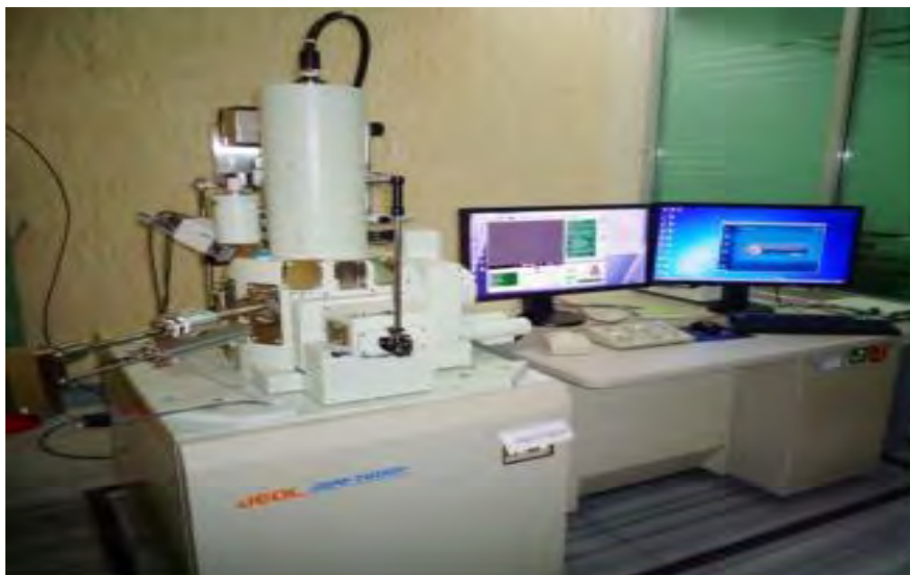
Fig. 18: FESEM setup for taking images of NPs
