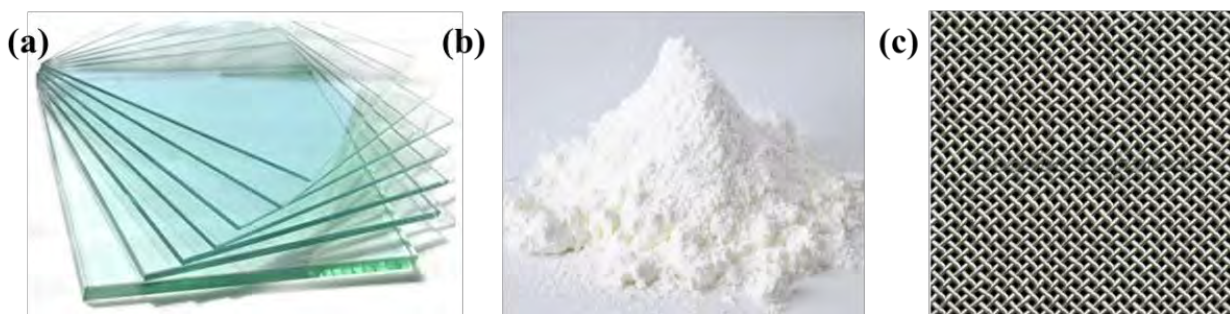
Figure 3.3: Immobilizing materials (a) Borosilicate glass, (b) White cement, and (c) Steel wire mesh
