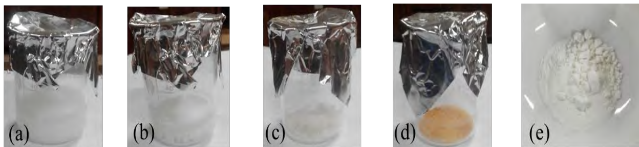
Figure 3.1: Heat treatment procedure from gel to \text{TiO}_2 nanoparticle; (a) Sol-gel of \text{TiO}_2 after 12-hour aging (b) Heat treatment of 1 hour at 90^\circ\text{C} (c) Heat treatment of 1 hour at 100^\circ\text{C} (d) Heat treatment of 1 hour at 110^\circ\text{C} and (e) Heat treatment of 4 hours at 400^\circ\text{C} and 500^\circ in a muffle furnace.
