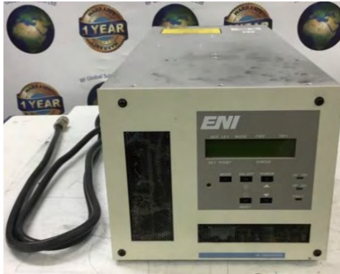
Fig. 3.4: A photograph of a RF Generator.
