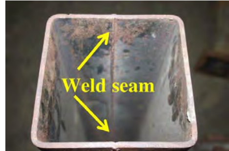
(b) Square cross-section of hollow built-up steel tube
