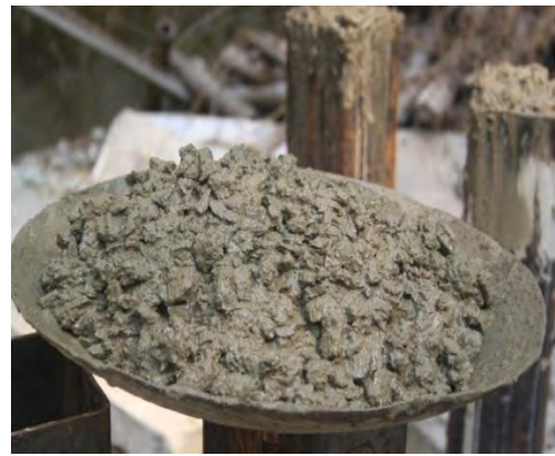
(b) Fresh Concrete
