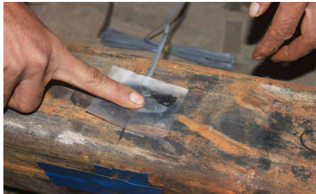
(a) Installation of strain gauge
