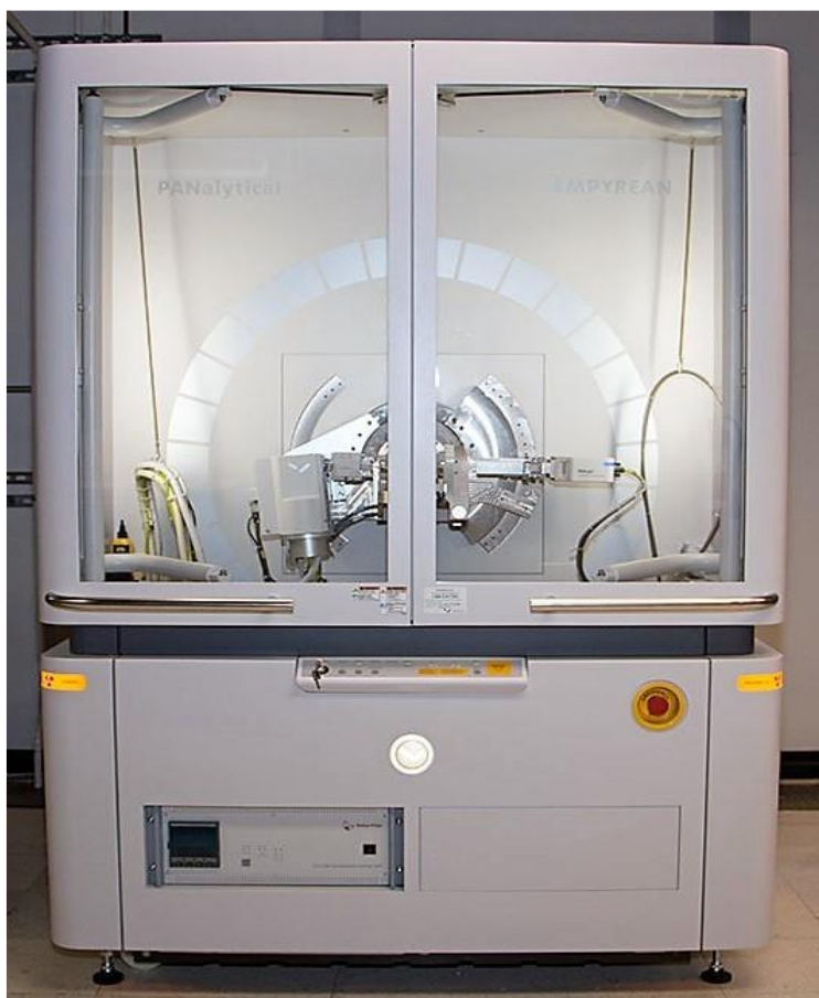
Figure 3.8: X-ray diffractometer set up.
