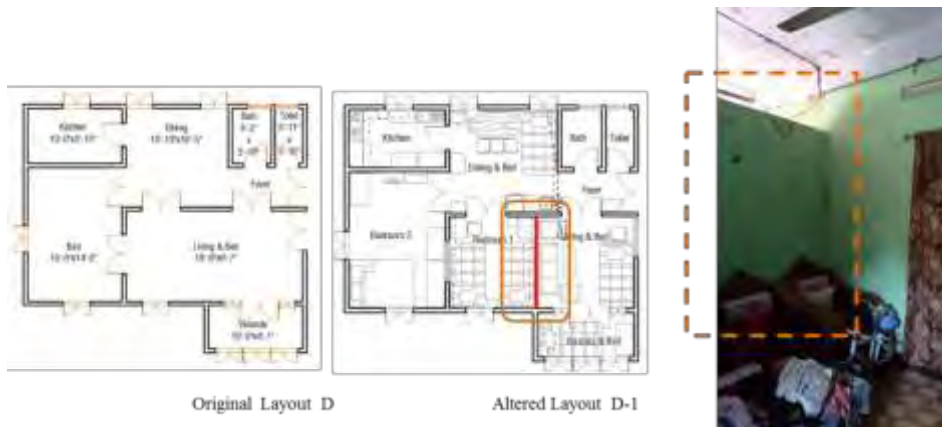
Fig 3.21: Use of Partition wall, sample D-1
