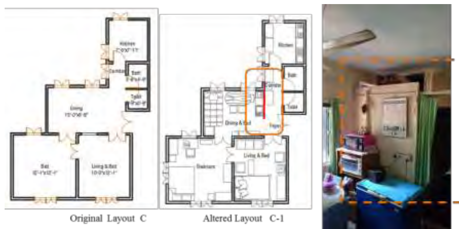
Fig 3.22: Use of Partition wall, sample C-1
