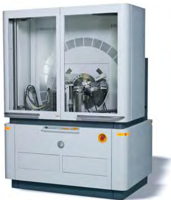
Fig. 4.3: A typical X-ray diffractometer used for XRD [5].
