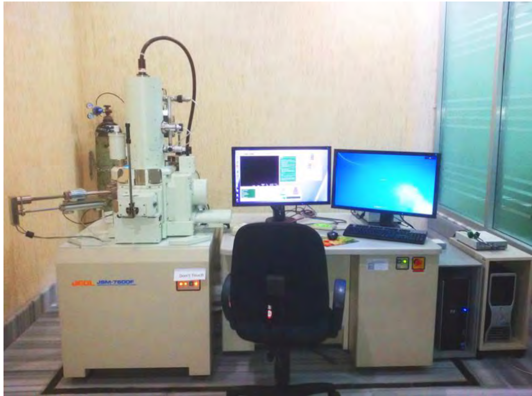
Fig. 4.5: Field emission scanning electron microscope (FESEM) setup.
