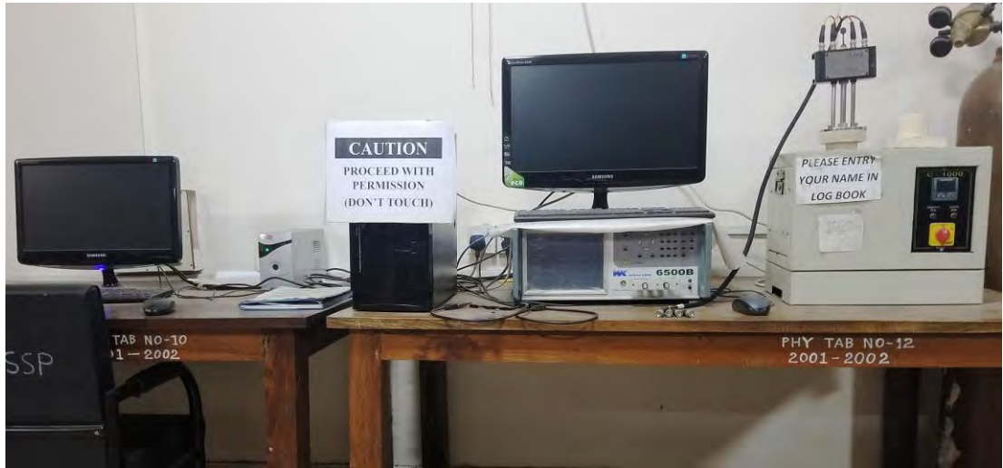
Fig. 4.8: Experimental setup of Wayne Kerr Impedance Analyzer (6500B).
