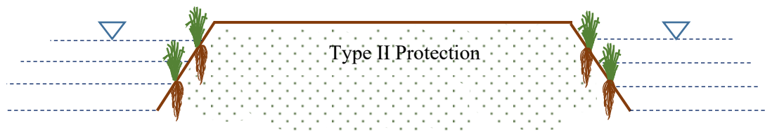
Figure 3.27: Schematic View of Killa Protection
