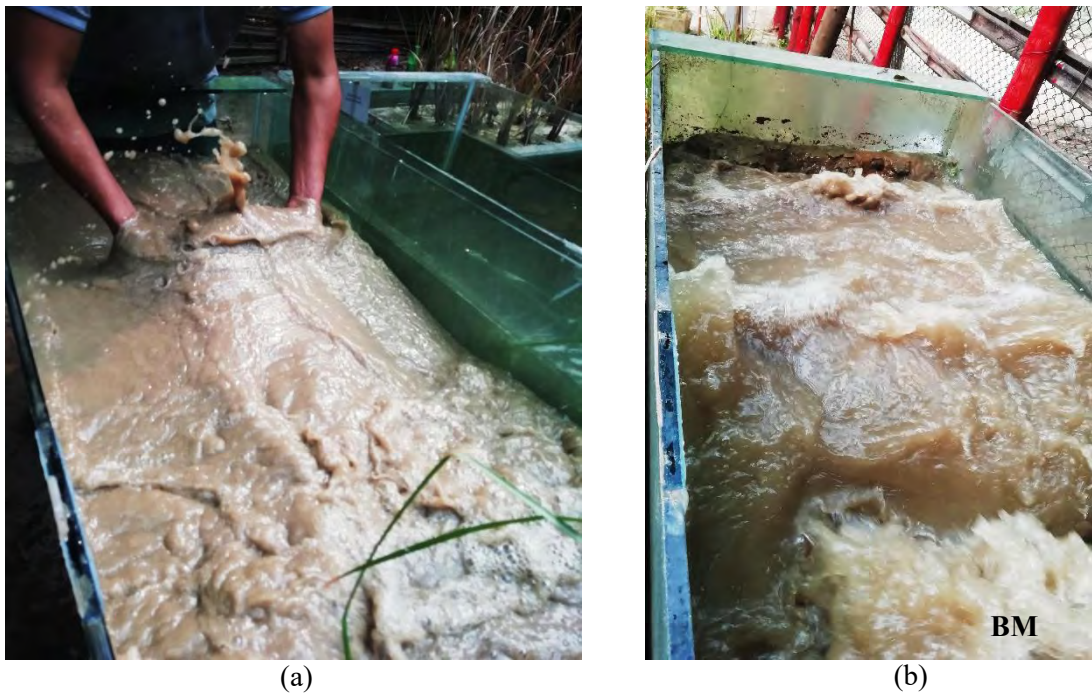
Figure 3.10: (a) Wave Action Propagation; and (b) Huge Wave Generation at Model BM
