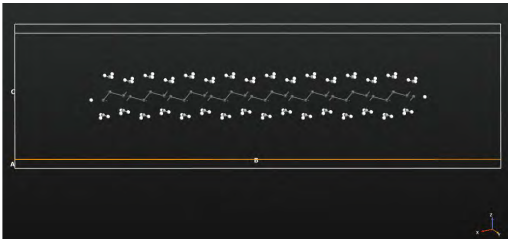
Figure 2.4 Initial frame for molecular dynamics simulation of PbCH 3 monolayer. The CH 3 groups are released to become attached to lead atom sites.
