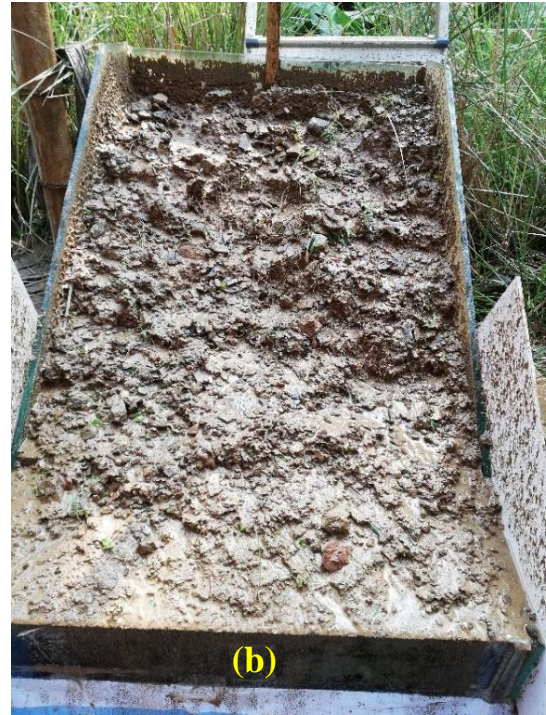
Figure 4.11: (a) Eroded soil with runoff; (b) Eroded surface after rainfall of M-6
