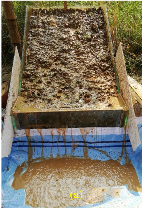
Figure 4.11: (a) Eroded soil with runoff; (b) Eroded surface after rainfall of M-6
