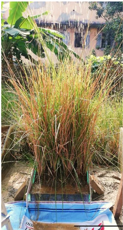
Figure 4.12: Rainfall test on M-1 generating low sediment yield
