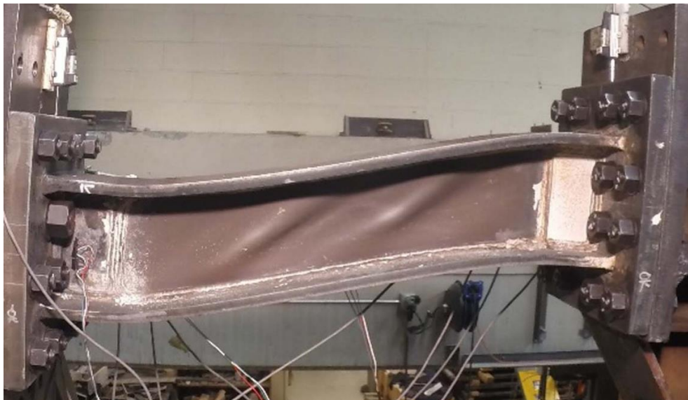
Figure 4.17: Deformed shape of specimen AL-BU-B2 (Volynkin et al. 2018)
