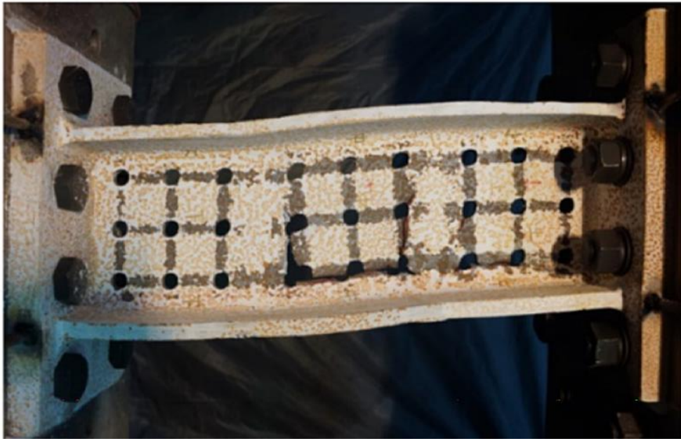
Figure 4.28: Deformed shape after failure of L-C-1 (at -0.07 radian rotation) (Tong et al. 2018)
