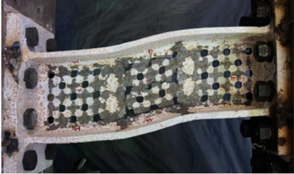
Figure 4.30: Deformed shape after failure of L-C-2 (at 0.11 radian rotation) (Tong et al. 2018)
