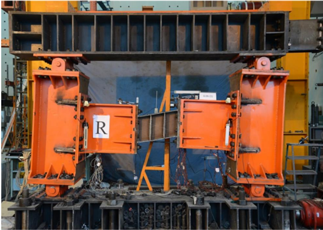
Figure 2.20: Schematic view and test setup of replaceable coupling beam with shear link (Ji et al. 2017)
