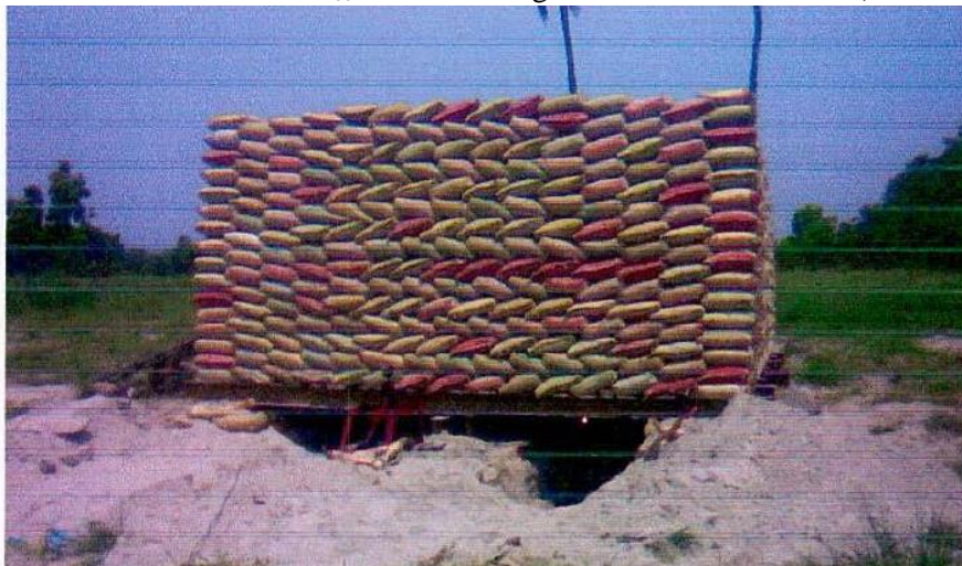
Figure 3.5: Photograph of a pile static load test
