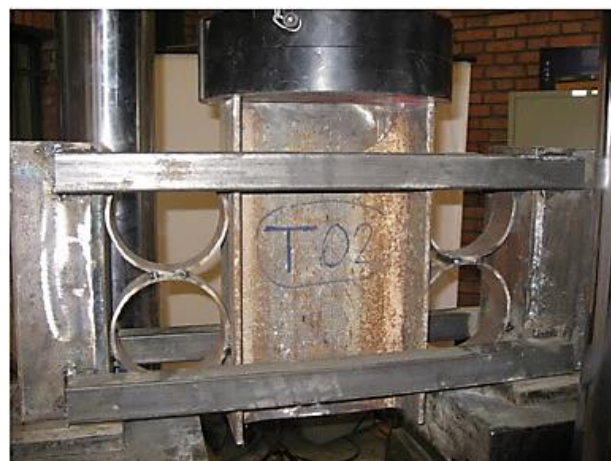
Fig. 2.21: Dual-pipe damper (Maleki and Mahjoubi 2013)
