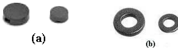
Figure 4.1: a. Pellets and b. Toroids shaped samples.
