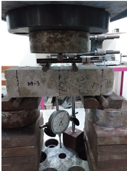
Figure 3-12 Flexural strength test on sample (before)
