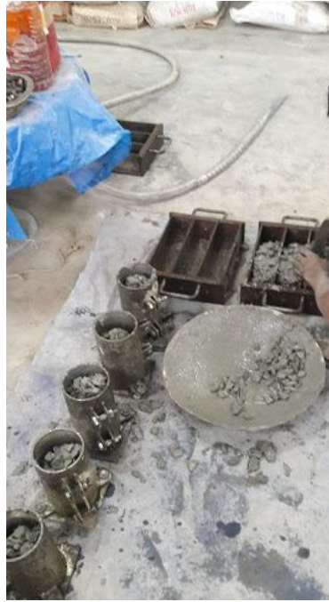
Figure 3-8 Concrete pouring in the molds
