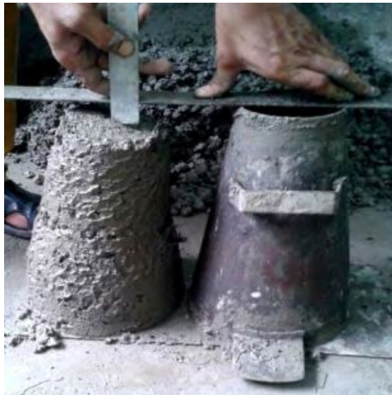
Figure 3-7 Slump value measurement
