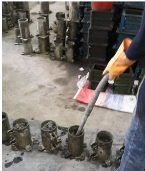
Figure 3-9 Compaction of concrete
