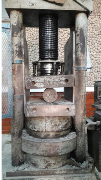
Figure 3-11 Splitting tensile strength test on sample
