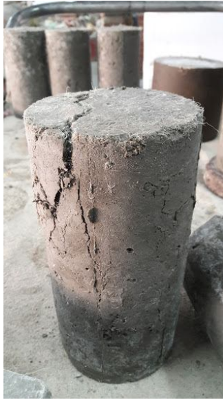
Figure 4-4 Sample after the compressive strength test (1)
