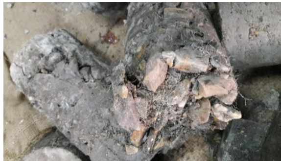
Figure 4-5 Sample after the compressive strength test (2)
