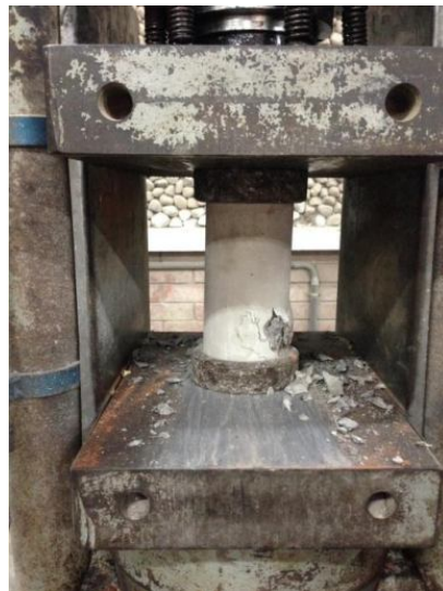
Figure 3-10 Machine used for compressive strength test
