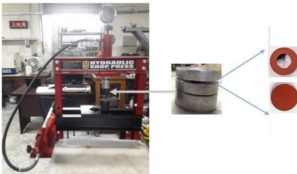
Fig.3.6: The pelletization in the form of pellet/disc and toroid in step-4
