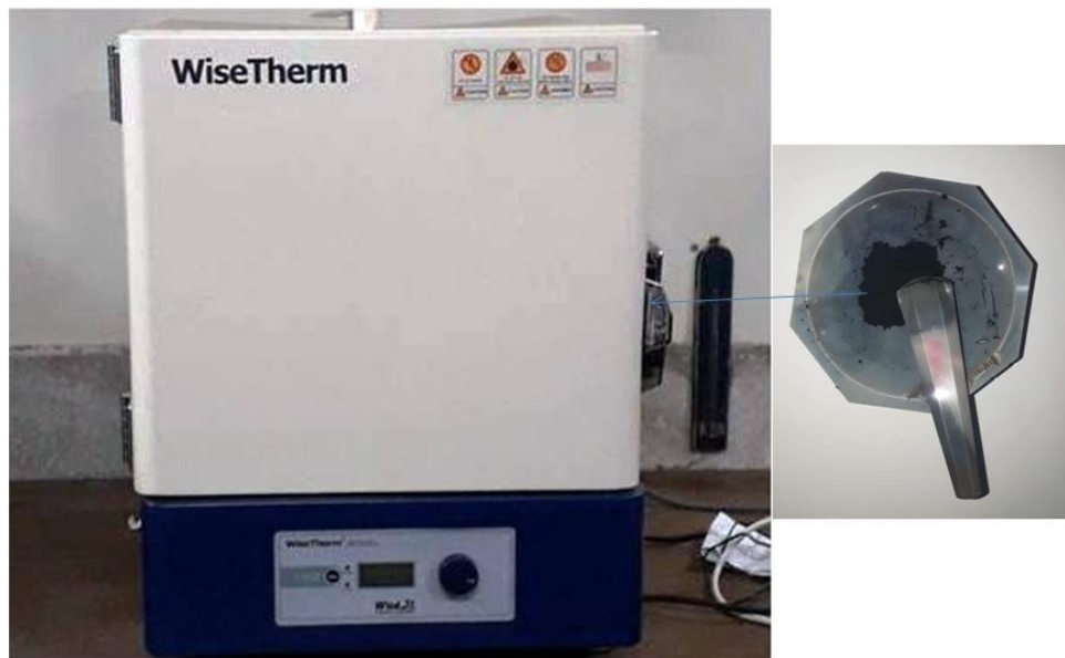
Fig.3.5: WiseTherm Furnace used for the calcination of the ball-milled powders in step-3
