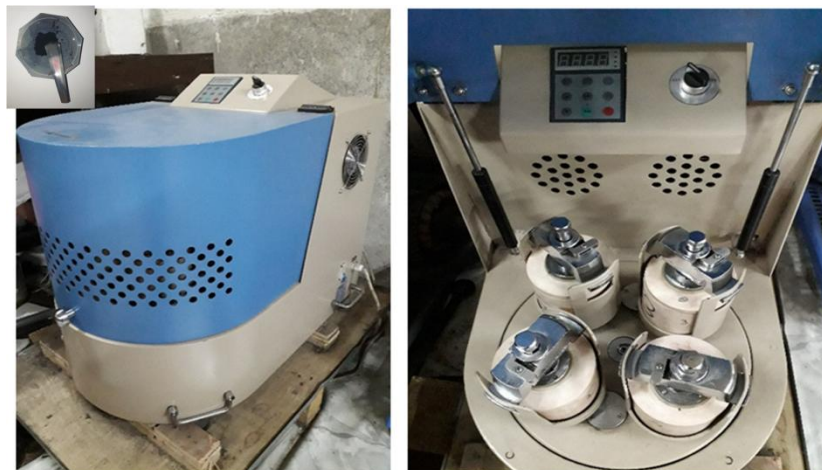
Fig.3.2: Ball mill and its cross-section picture(MSK-SFM-1benchtop planetary ball mill)-step-1-2
