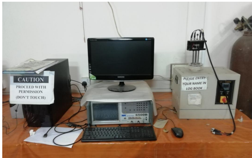
Fig. 3.24 Experimental setup of Wayne Kerr Impedance Analyzer (6500B).
