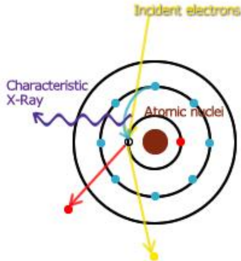
Fig. 3.21 Characteristic X-ray Generation Process.
