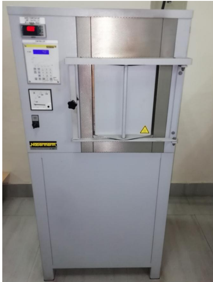
Fig.3.8 Typical diagram of a programmable electric furnace.
