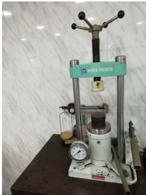
Fig. 3.10 Typical diagram of a Hydraulic press.
