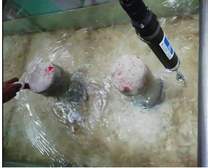
Figure 3.9: Wake is generating between two cylinders
