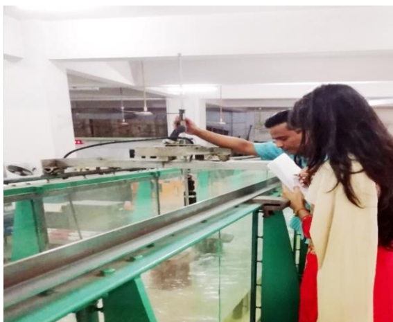
Figure 3.13: Changing the position of ADV for different sections
