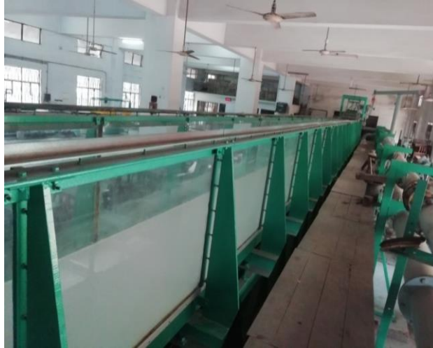
Figure 3.1: Laboratory flume (21.3 m long, 0.76 m wide and 0.74 m deep)
