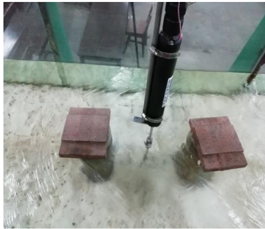
Figure 3.10: Laboratory set-up of velocity measuring locations
