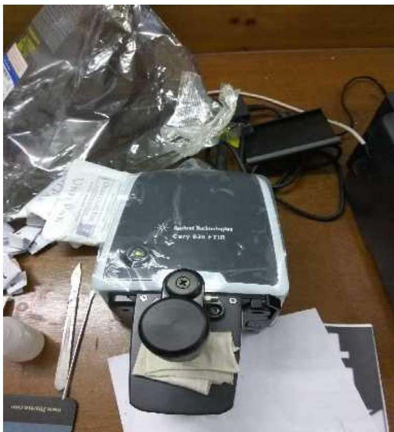
Fig 3.2: Cary 630 FTIR by Agilent Technologies
