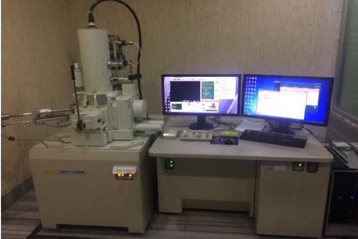
Fig 3.3: JEOL JSM-7600F Scanning Electron Microscope (SEM)
