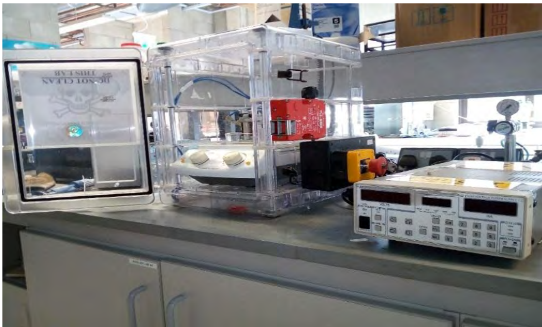
Figure-3.6: High voltage power supply and desiccators box with locking mechanism
