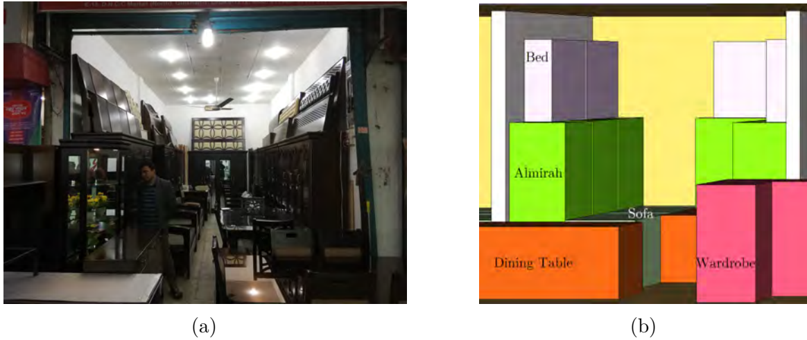
Fig. 2.16 (a) Photographed furniture fuel arrangement in DCC market. (b) Five types of furniture designed in Pyrosim and arranged according to real arrangement. Different types of furniture were assigned different color and labeled here. The color always represents the same furniture type throughout the study.
