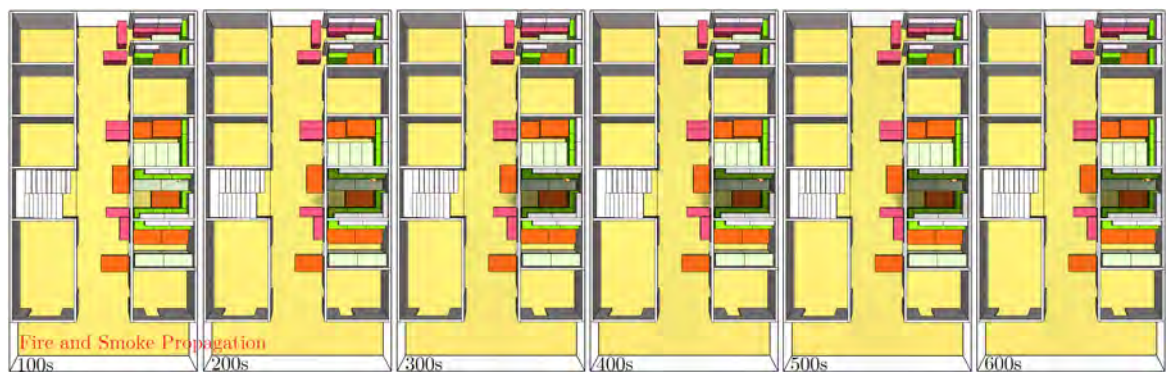
Fig. 3.23 Flame propagation through DCC market source shop 1, DCC_FS1, in case of furniture as fuel load. The figure shows both flame and smoke for 100s, 200s, 300s, 400s, 500s and 600s of simulation time respectively from left to right.
