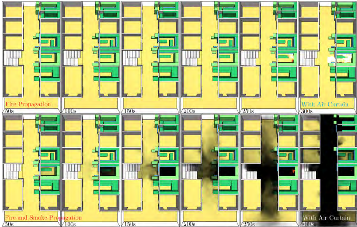
Fig. 3.60 Flame propagation through DCC market source shop 1, DCC_CS1AC, in case of clothing as fuel load, with a vertical air curtain of 7.62 cm jet width and 10 m/s jet velocity. The top row shows the flame propagation only, and bottom row shows both flame and smoke propagation for 50s, 100s, 150s, 200s, 250s and 300s of simulation time respectively from left to right.
