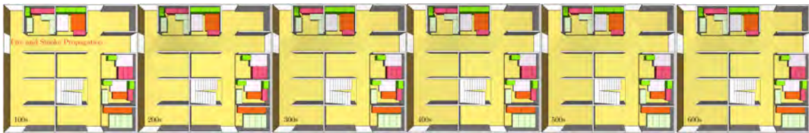
Fig. 3.45 Flame and smoke propagation through Co-Operative market source shop 2, CoOp_FS2, in case of clothing as fuel load. The figure shows both flame and smoke for 100s, 200s, 300s, 400s, 500s and 600s of simulation time respectively from left to right.
