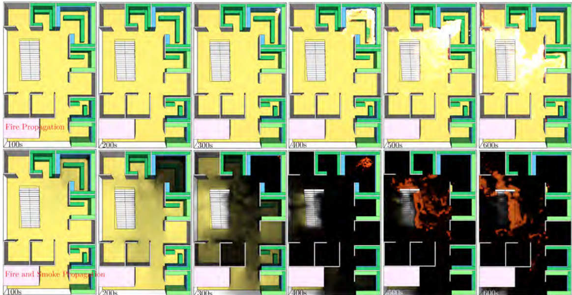
Fig. 3.52 Flame propagation through MultiPlan shopping complex source shop 1, MP_CS1, in case of clothing as fuel load. The top row shows the flame only, and bottom row shows both flame and smoke for 100s, 200s, 300s, 400s, 500s and 600s of simulation time respectively from left to right.
