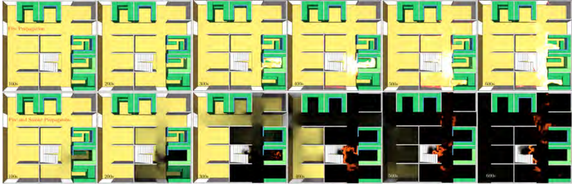
Fig. 3.36 Flame propagation through Co-Operative market source shop 1, CoOp_CS1, in case of clothing as fuel load. The top row shows the flame only, and bottom row shows both flame and smoke for 100s, 200s, 300s, 400s, 500s and 600s of simulation time respectively from left to right.
