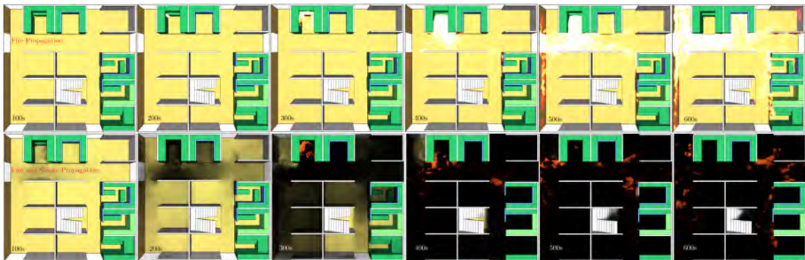
Fig. 3.37 Flame propagation through Co-Operative market source shop 2, i.e., for CoOp_CS2 simulation, in case of clothing as fuel load. The top row shows the flame only, and bottom row shows both flame and smoke for 100s, 200s, 300s, 400s, 500s and 600s of simulation time respectively from left to right.
