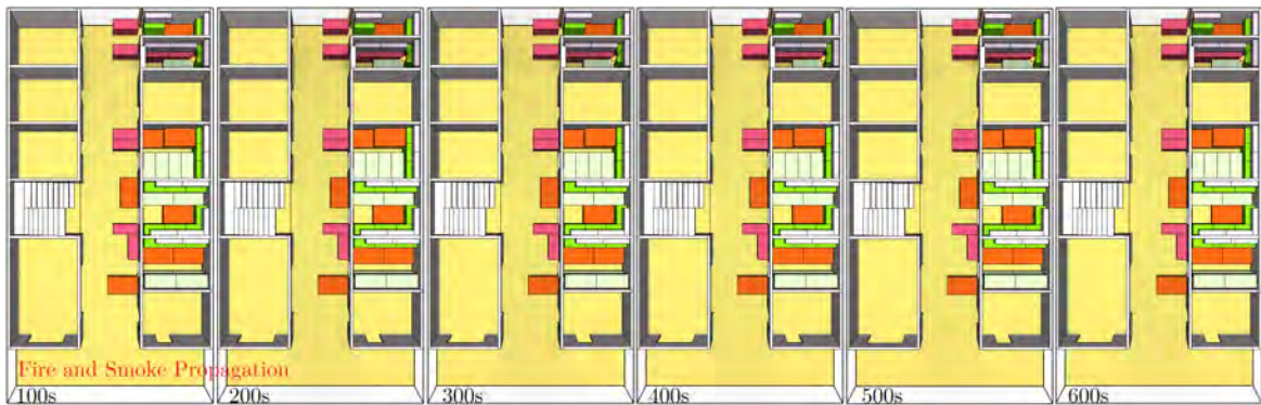
Fig. 3.27 Flame propagation through DCC market source shop 2, DCC_FS2, in case of clothing as fuel load. The figure shows both flame and smoke for 100s, 200s, 300s, 400s, 500s and 600s of simulation time respectively from left to right.
