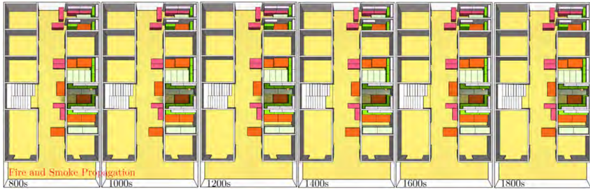
Fig. 3.24 Flame propagation through DCC market source shop 1, DCC_FS1, in case of furniture as fuel load. The figure shows both flame and smoke for 800s, 1000s, 1200s, 1400s, 1600s and 1800s of simulation time respectively from left to right.
