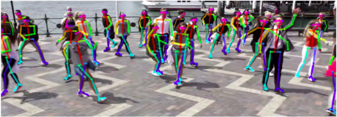
Figure 3.12: Realtime multi-person 2D pose estimation using OpenPose algorithm. [Image courtesy Cao et al. [26]]
