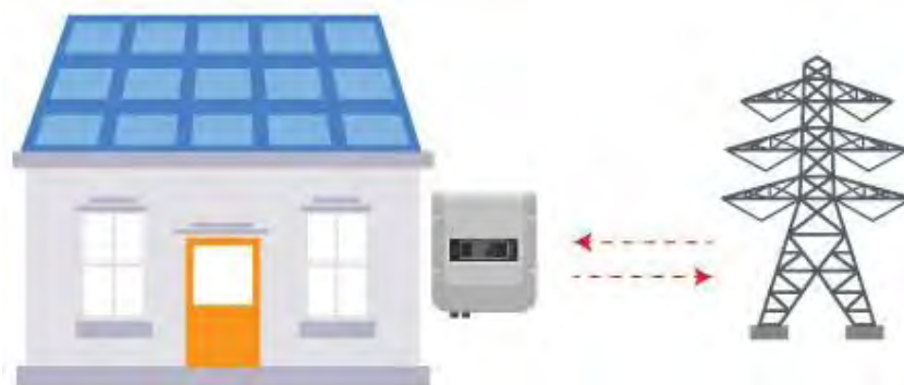
Figure 2.3: Grid tied solar system.
