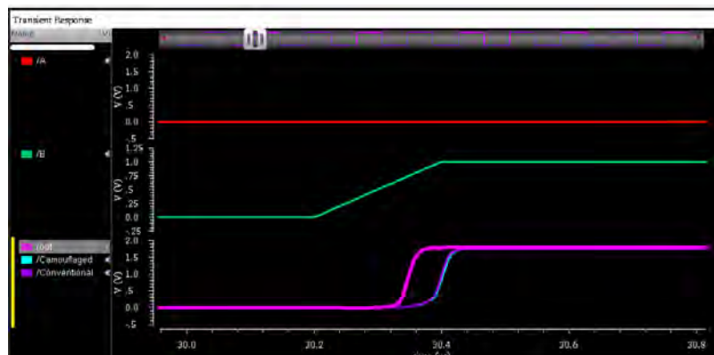
Figure 3.6: Delay due to RC Extraction.
