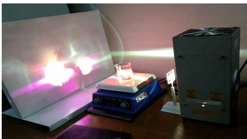
Figure 3.7 Photocatalytic activity measurement setup with Xenon lump housing E10180
