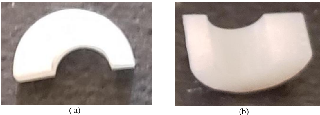
Figure 2.4 The sectioned samples for measuring the roughness at the interface between Ti and Cement: (a) longitudinal section view and (b) transverse section view.
