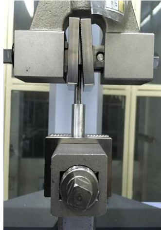
Figure 5.2 Fatigue test on a Ti/Cement samples in the UTM.
