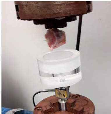
Figure 4.1 Mechanical stability tests on a titanium/bone sample.
