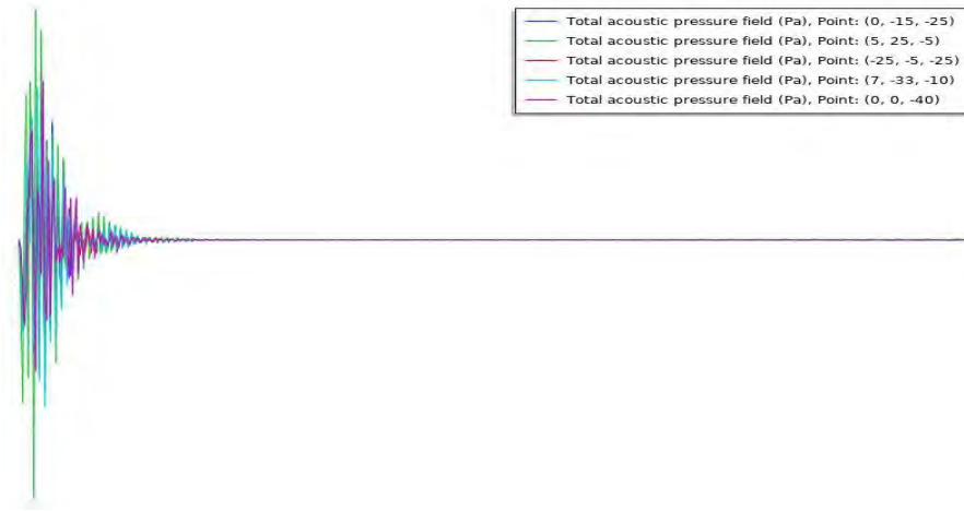
Figure 6.2: Acoustic field pressure on output Probe points Vs. Time [0-10 sec] of reduced order Piezo Tonpilz Transducer
