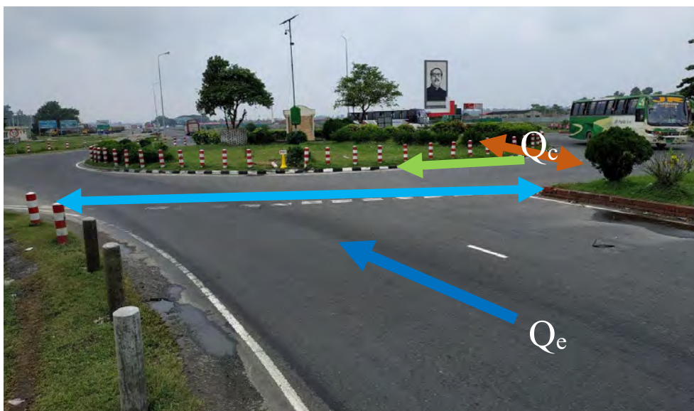
Figure 3.9 Measurement Position of entry flow ( Q_e ) and circulating flow ( Q_c )
