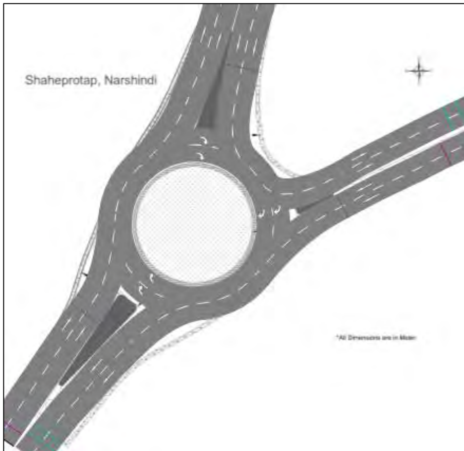
Figure 5.16 VISSIM model coding of roundabout R6
