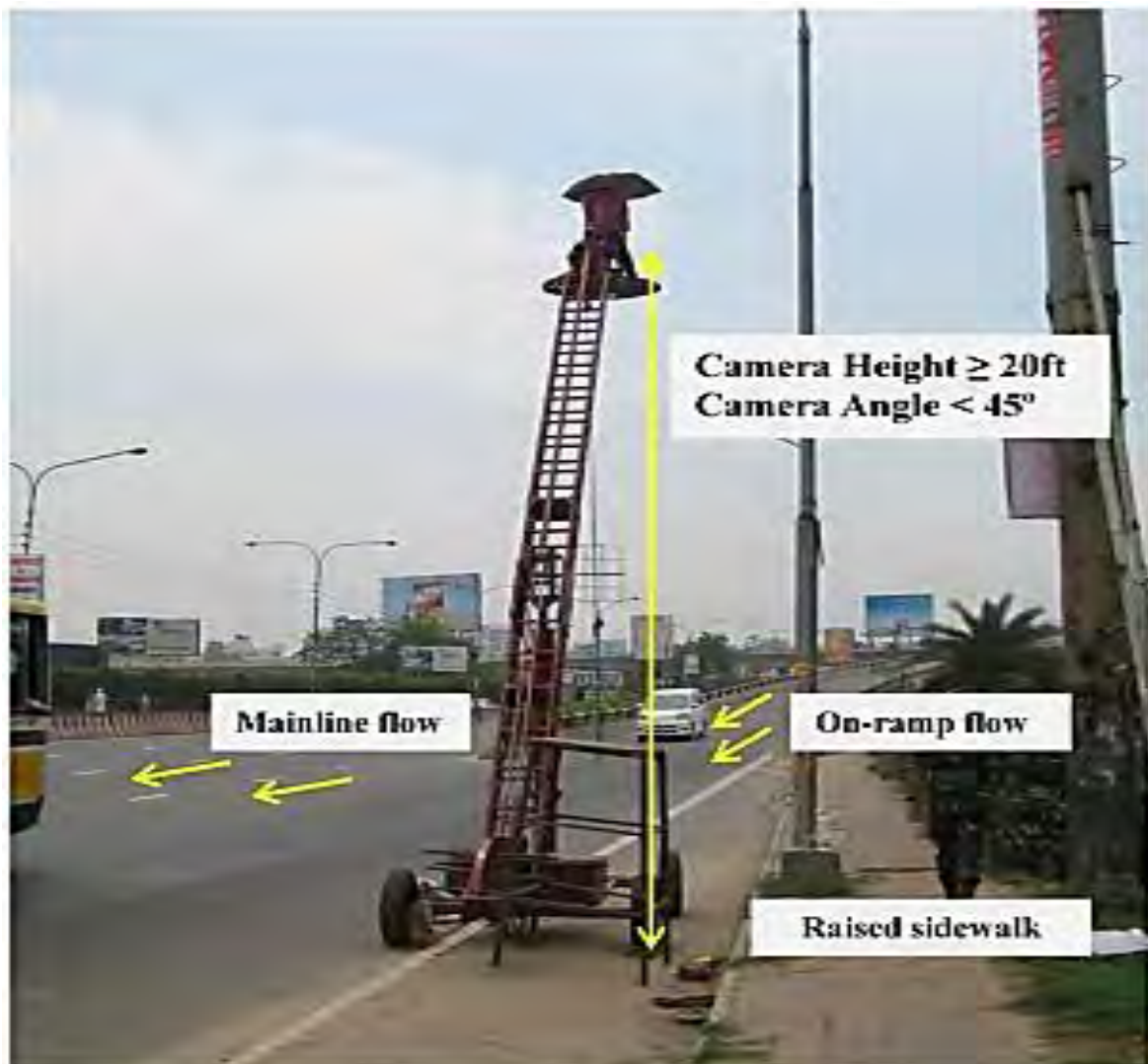
Figure 4:3 Detailing of camera setting for data collection
