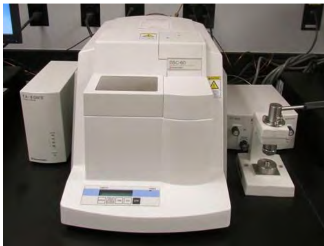
Figure 3-1: Differential scanning calorimetry (DSC-60, Shimadzu, Japan)
