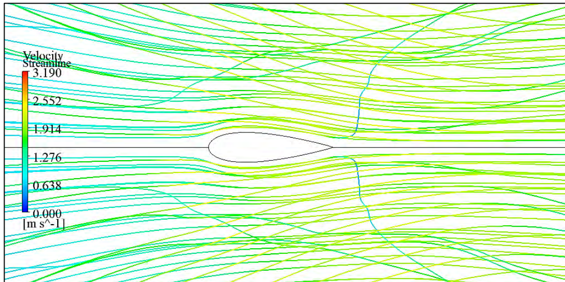
Figure 4.10.9: Streamline along NACA 0024 airfoil section with Fr = 0.55
