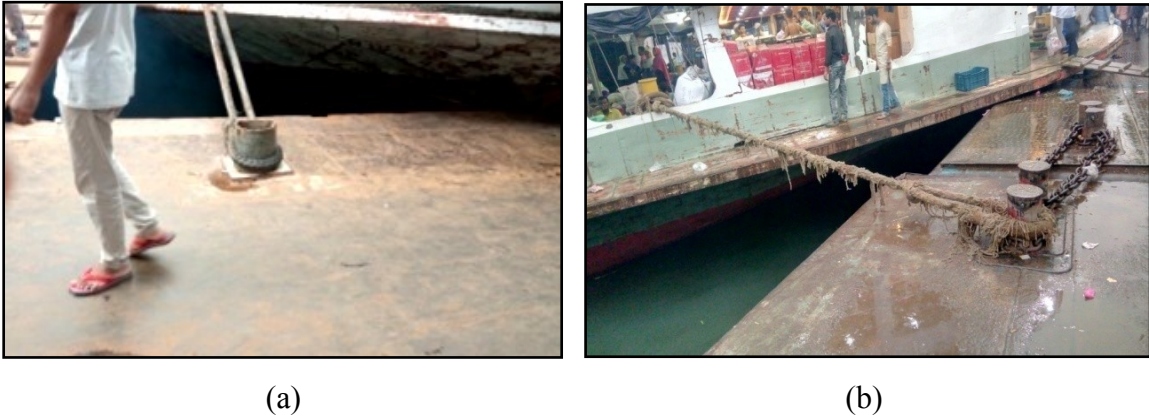
Fig. 5.7: (a) Unchecked condition of a mooring rope that is under huge tension; (b) Worn out condition of mooring rope, source: author.
