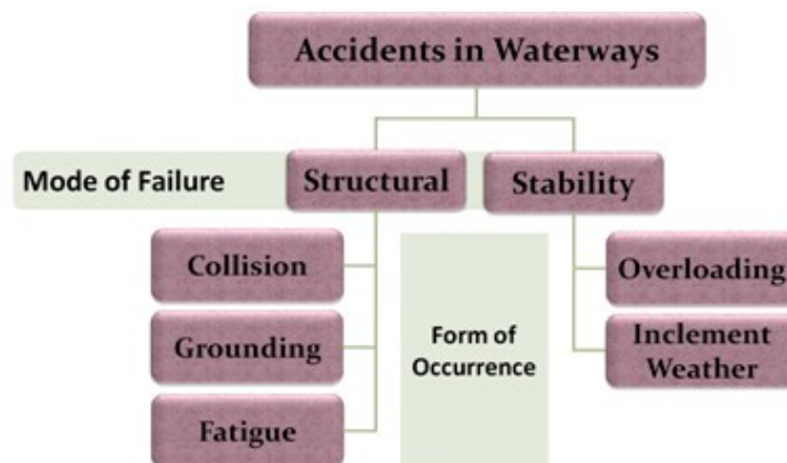
Fig. 2.8: Mode of failure and form of occurrences of accidents in the waterways, reproduced from Islam et al. (2015).
