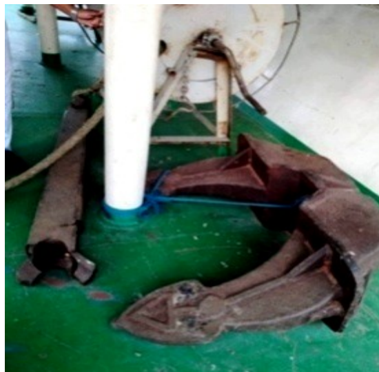
Fig. 5.11: A broken anchor in an inland passenger ship, source: author.
