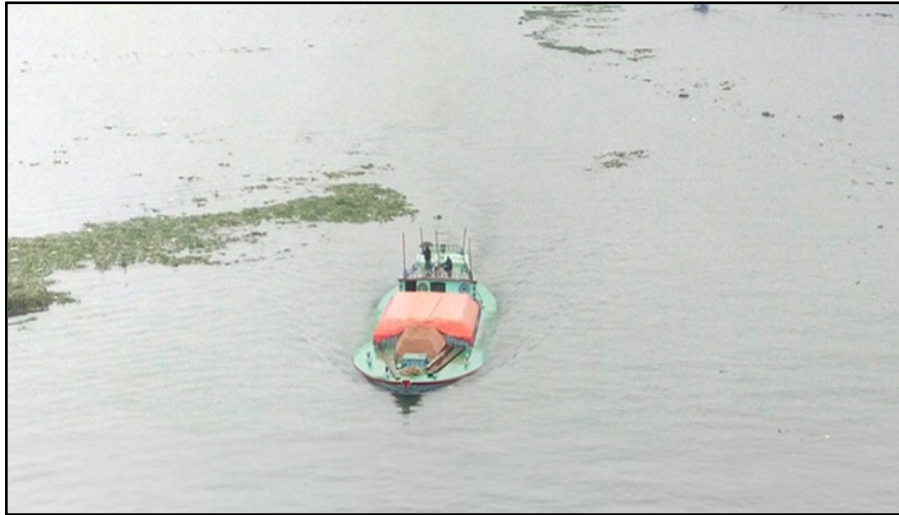
Fig. 2.3: Movement of a 'Bulkhead' in the overloaded condition, source: author.
