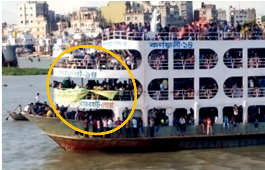
Fig. 5.12: Extended portion of the bridge deck and upper deck that creates visual obstruction during mooring operation, source: author.
