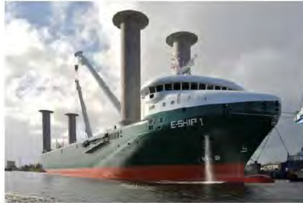
Figure 72: Magnus effect and E-ship 1[52]
