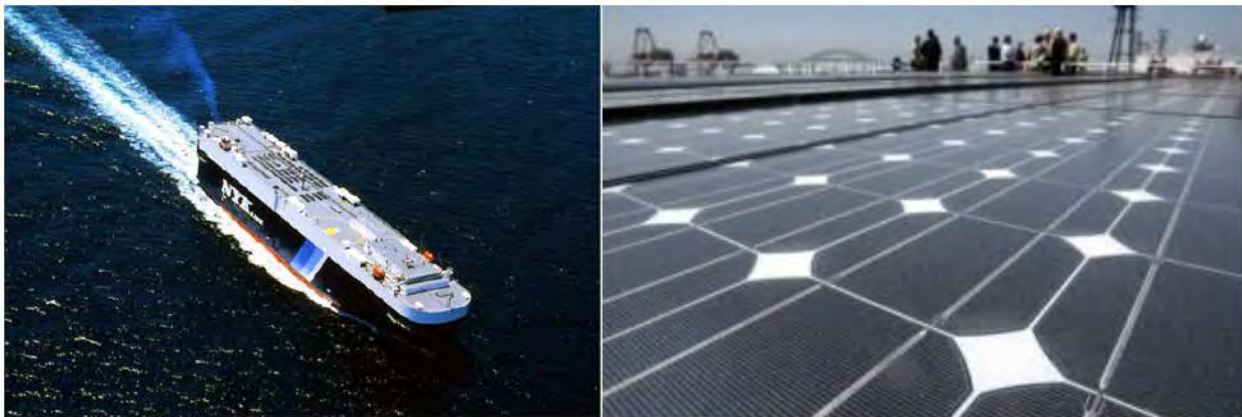
Figure 73: MV Auriga Leader (left) with solar panels (right) installed on deck
