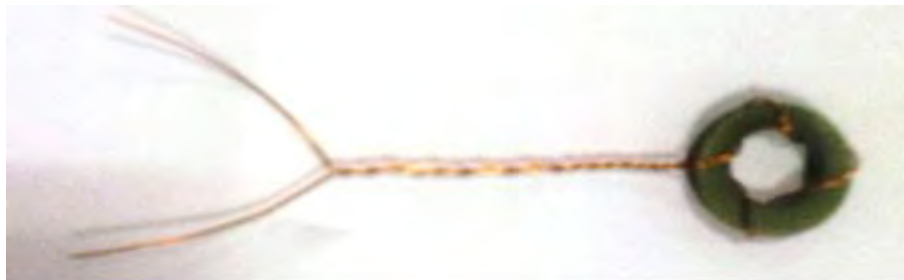
Fig. 3.10 Toroid shaped sample for the measurement of permeability.
