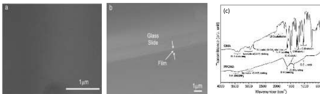
Fig. 2.4: The SEM micrographs: (a) slide view, and (b) cross sectional view of the PPOMA thin films, (c) The FTIR spectra of OMA and PPOMA [26].
