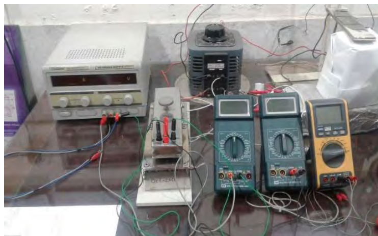
Fig. 3.27 Four point probe set up: Optical microscopy lab, Department of Physics, BUET.
