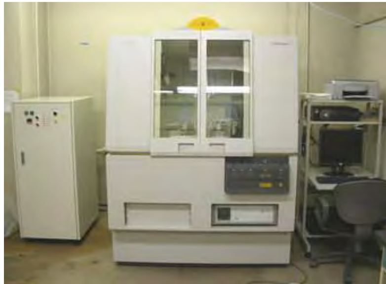
Fig. 3.20 X-ray diffractometer (XRD); model: PANalytical Empyrean series 2.
