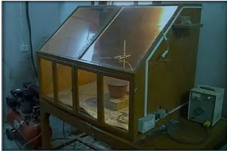
Fig. 3.14 Setup of spray pyrolysis technique (Department of Physics, BUET).
