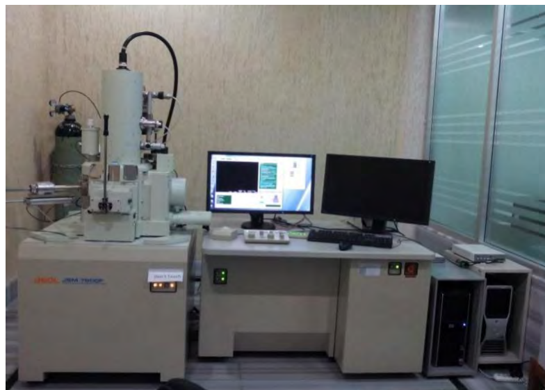
Fig. 3.16 Field emission scanning electron microscope, model: JEOL JSM-7600F.
