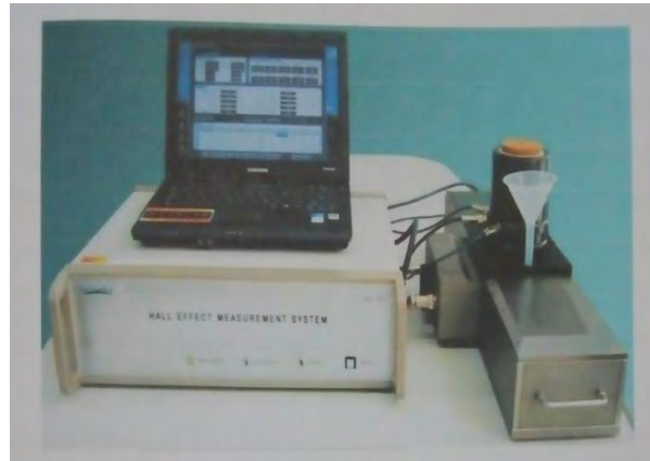
Fig. 3.29 Hall effect measuring apparatus (ECOPIA HMS-5000, USA).
