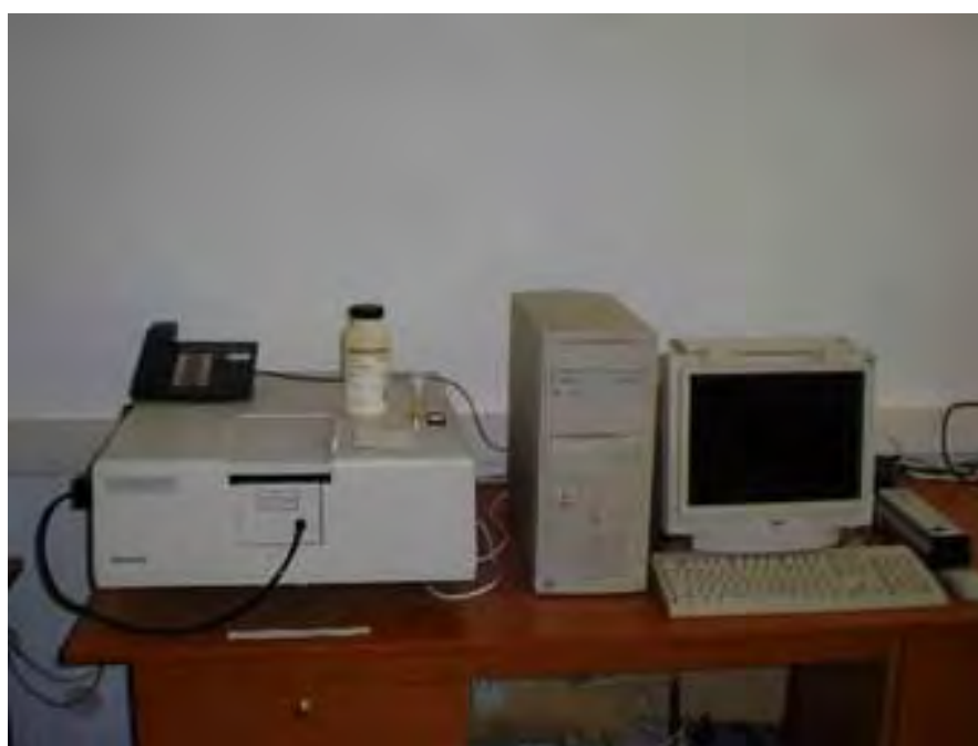
Fig. 3.22 UV-Vis spectrophotometer (Model: UV-2600, Pc:UV-Vis-NIR; Shimadzu).
