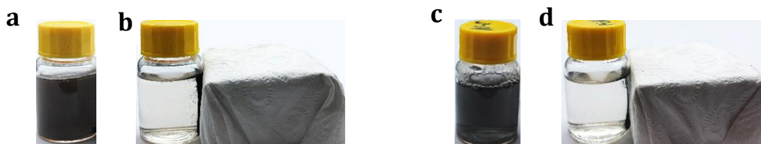
Figure 3.7 (a) Initial state of \text{Fe}_3\text{O}_4 -PD-NIPAm-co-AMPS submicrometer-sized hydrogel particles (b) After 50 seconds of applying magnetic force (c) Initial state of Ni-PD-NIPAm-co-AMPS (d) After 50 seconds of applying magnetic force
