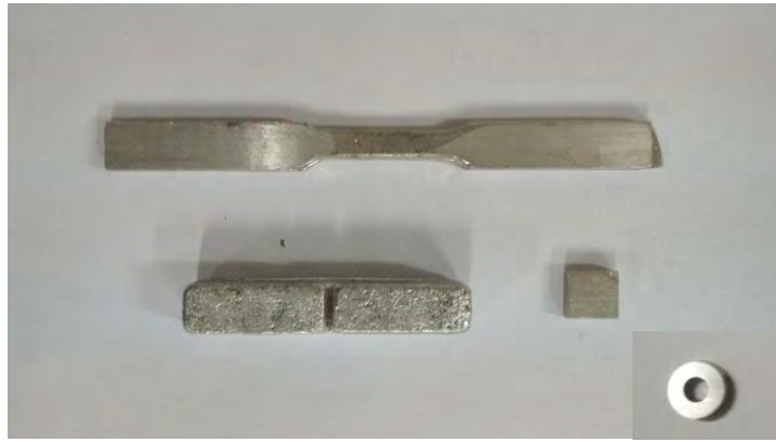
Figure 3. 3 Actual photographs of mechanical, electrical and magnetic test samples
