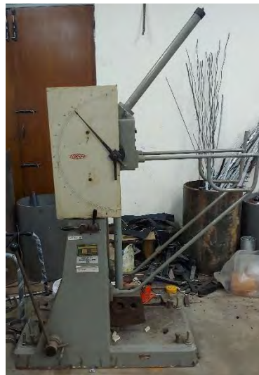
Figure 3. 6 Charpy impact tester
