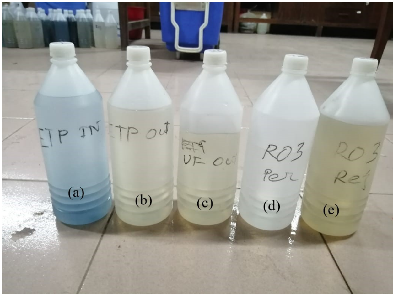
Figure 4.15: (a) Wastewater (b) ETP treated water (c) UF reject water (d) RO permeate and (e) RO reject water for the washing factory 1
