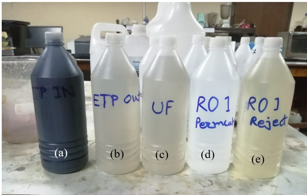
Figure 4.12: (a) Wastewater (b) ETP treated water (c) UF reject water (d) RO permeate and (e) RO reject water for the woven dyeing factory 1
