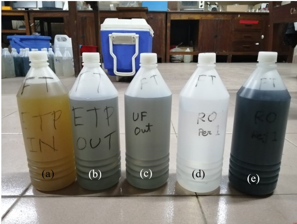
Figure 4.8: (a) Wastewater (b) ETP treated water (c) UF reject water (d) RO permeate and (e) RO reject water for the knit dyeing factory 1
