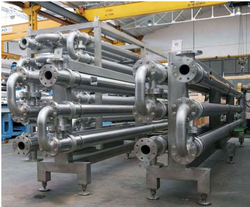
Fig. 1.1: Heat exchanger installed at a power plant.
