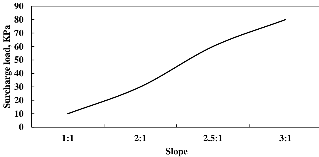
Figure 5.13: Variation of surcharge load with change in slope for initiation of bank failure
