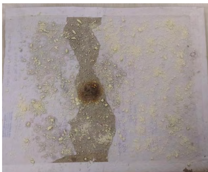
Fig. 3.4: Locating the hot spot position within the microwave chamber, the exact hotspot location on the hard paper board.
