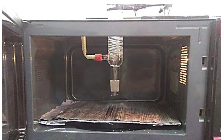
Fig. 3.3: Placement of hard paper board at proper height.
