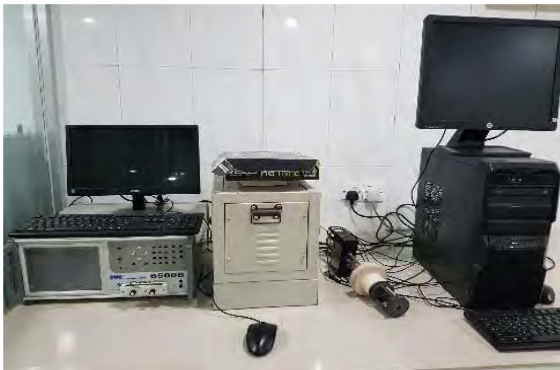
Fig. 3.12: The dielectric property was measured using an impedance analyzer (Wayne Kerr, 6500B series).
