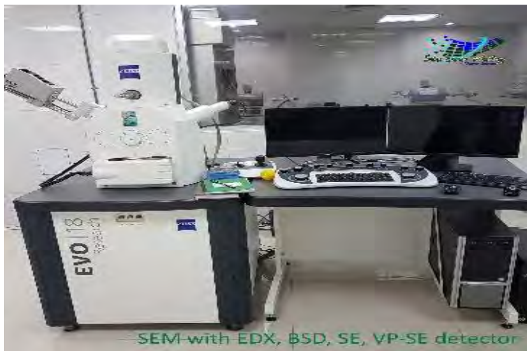
Fig. 3.9: Morphological and elemental analysis were done by an SEM with EDX (Carl Zeiss, EVO 18).
