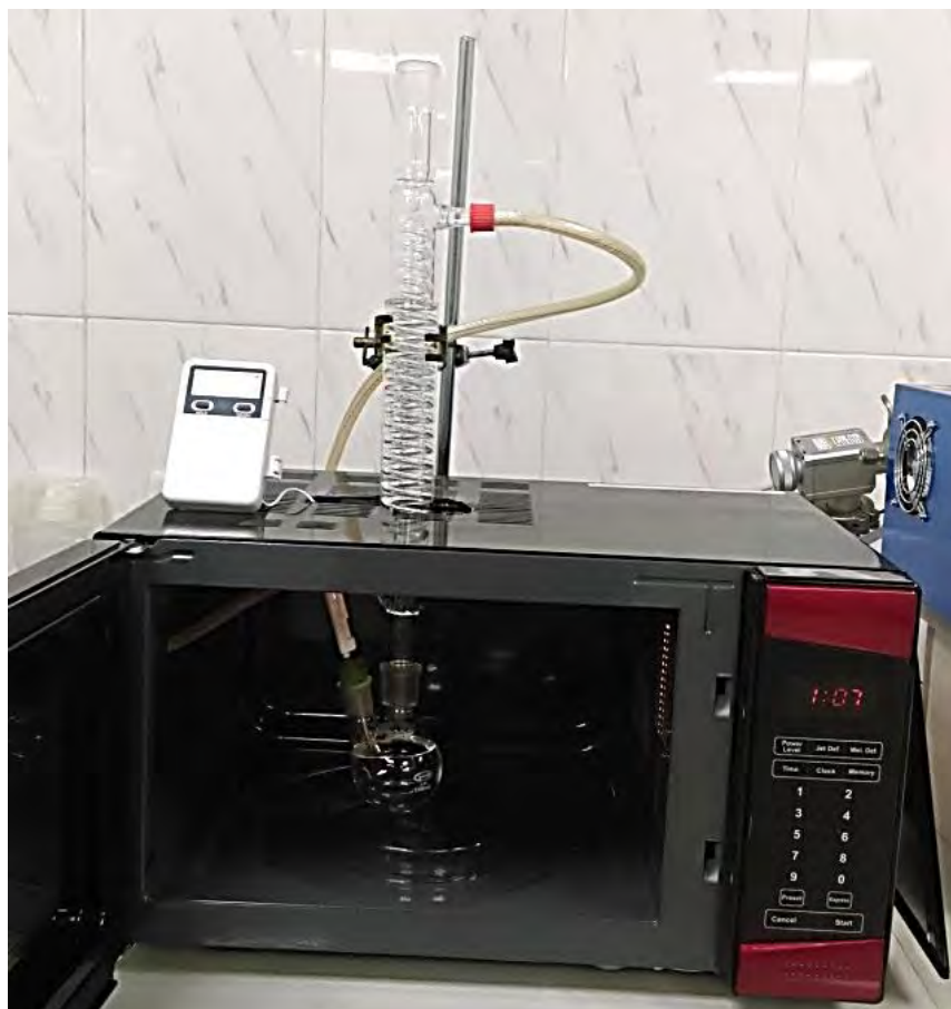
Fig. 3.2: Photograph of the customized microwave oven.
