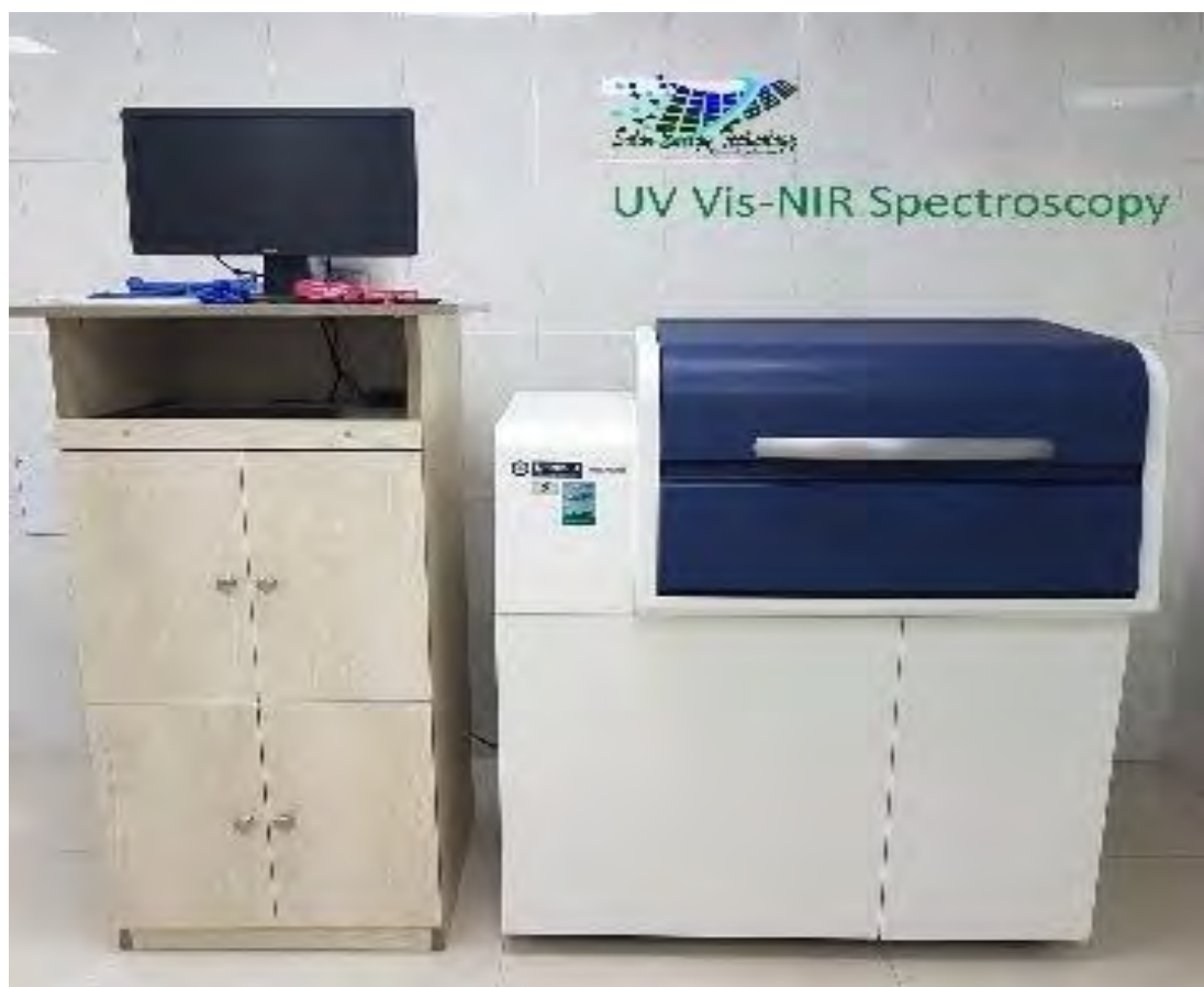
Fig. 3.11: The optical measurements were done using an UV-Vis-NIR (Hitachi, UH4150) spectrophotometer coupled with an integrating sphere.
