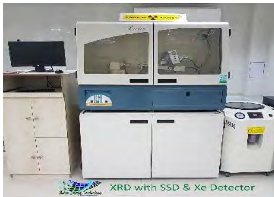
Fig. 3.8: The structural as well as phase identification measurements were carried out by an X-ray Diffractometer (GBC-XRD, EMMA) with a step size of 0.02 deg. using a \text{Cu\_K}\alpha_1 ( \lambda = 1.54062 \text{ \AA} ) radiation source operated at 35.5 kV and 28 mA.
